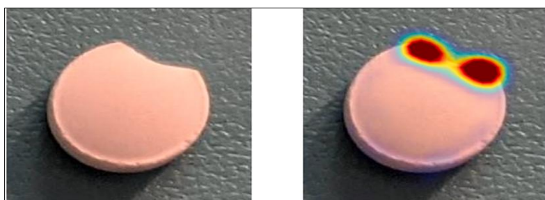
Fig 4: Detection of Tablet chipping using Neural networks
